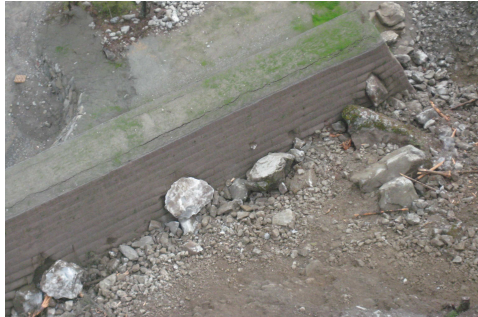
Valley side after impact – no displacements can be observed
